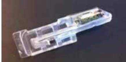
A translucent mini-skimmer made to sit (mostly) inside of an ATM's card acceptance slot. S
