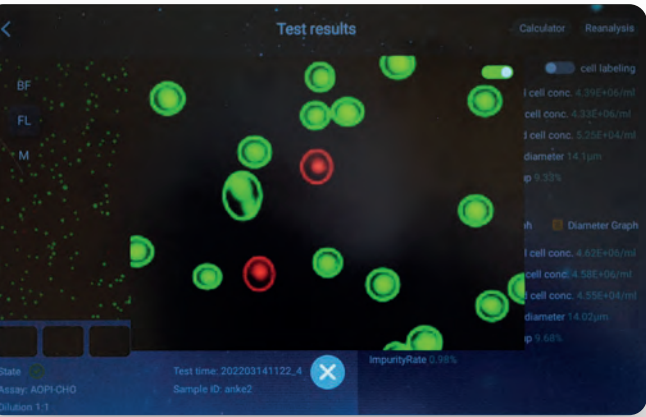
The same sample showing the fluorescence labelling results in an enlarged view – green circles identify the viable cells, red circles identify the dead or dying cells.
