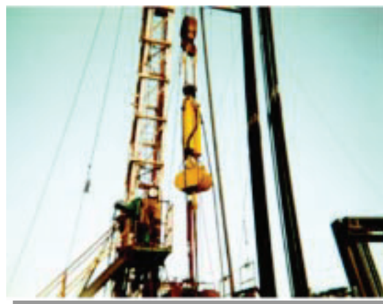
Vibration Technology Oscillator Used For Washover Pipe Recovery
