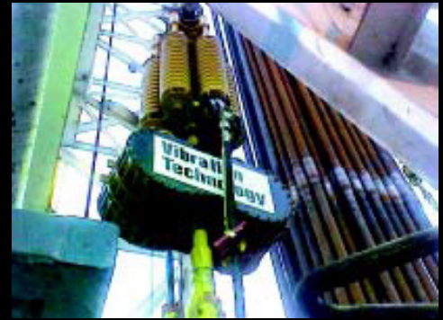
Vibration Technology's 500,000 lb working load oscillator makes quick work of freeing stuck pipe in drilling operations.
