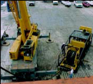
Hydraulic power drives Vibration Technology's surface oscillator.
