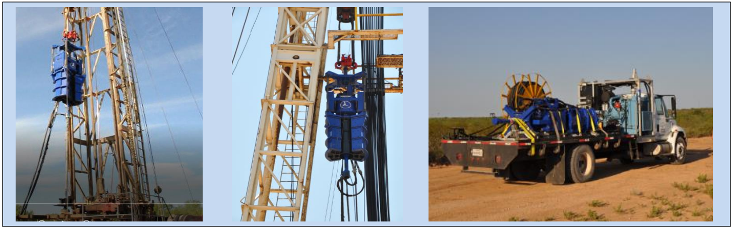
VIBRATION TECHNOLOGY RESONATOR EMPLOYING DOUBLE-ACTING HYDRAULIC PISTON/CYLINDER SINE WAVE GENERATOR
