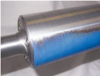
Roller after machine grinding— demonstrating exceptional adhesion and durability of Rilsan
