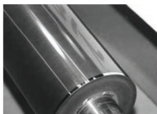
Water Pan Rollers with Ceramic coating (featuring stainless steel collars for edge protection)
