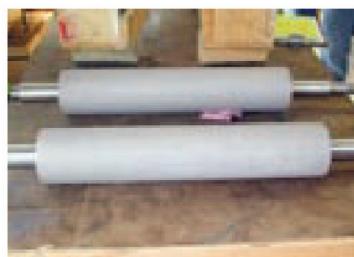
Draw Rolls with Tungsten Carbide Coating
