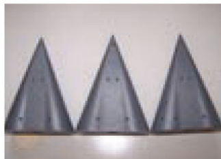
PFF Former Noses with Ceramic and High Release Coating
