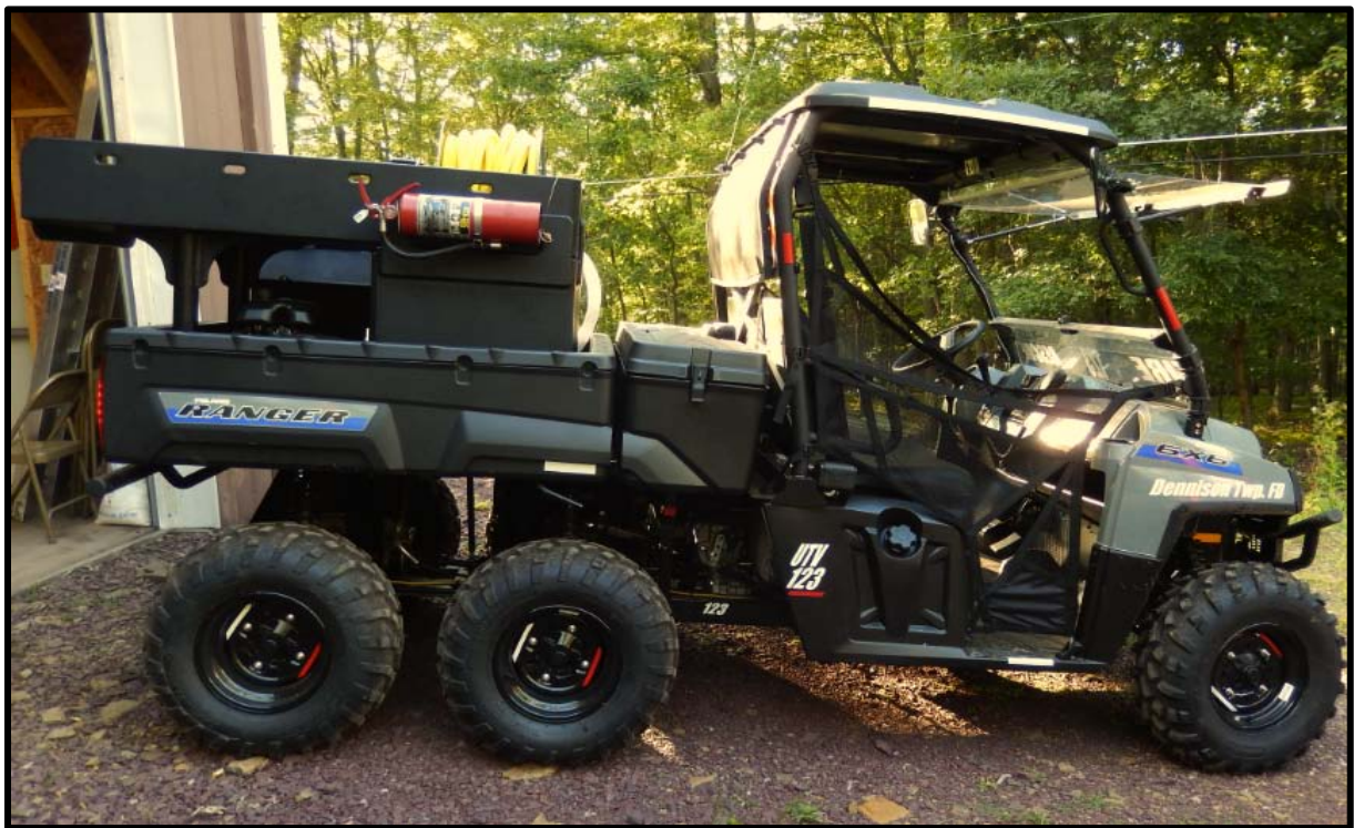
A 2014 Polaris Ranger Utility Vehicle, 6 wheel drive, with a “skid unit” equipped with a pump, a 100 gallon water tank, and a Stokes basket for rescues.
