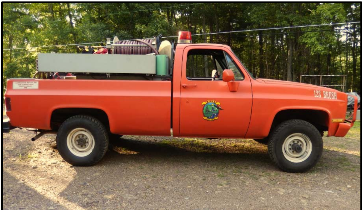
Brush Truck: 1986 Chevy ¾ ton pickup with a 200 gallon tank.
