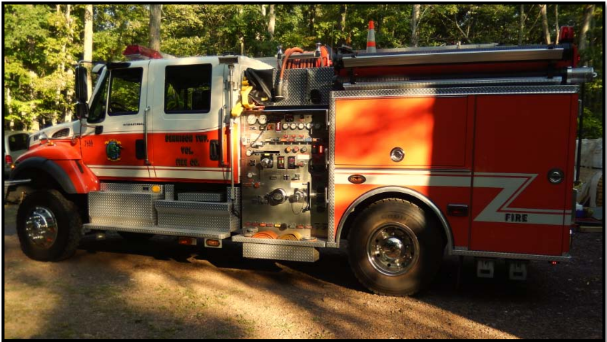
Engine 2; a 2005 Pumper with equipped four-wheel drive, a 750 gpm pump, and a compressed air foam system. In addition to firefighting equipment it carries Hurst hydraulic rescue tools. It is equipped with a 500 gallon water tank, 500 feet of 5 inch supply hose, a booster reel with 150 feet of 1½ inch attack line, three 1¾ inch attack lines, each 200 feet, and 200 feet of 2½ inch attack line.
