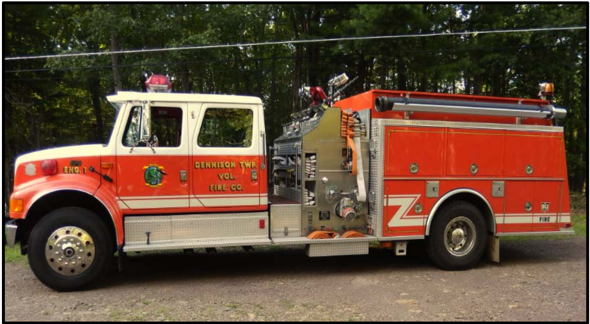
Engine 1; a 1996 KME Pumper with a 1,250 gpm pump, four 1\frac{3}{4} inch attack lines each 200 feet in length, two 2\frac{1}{2} inch attack lines each 200 feet in length, 1,000 feet of 5 inch supply line. It is equipped with a 1,000 gallon water tank and carries a battery powered hydraulic rescue tool.
