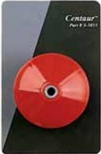
3035 Centaur® Centers the 9/32" hole in baluster bases for our Dowel-Fast screws. Fits 1-1/4" and 1-3/4" balusters. Doubles as a drill bit guide and a centering device.
