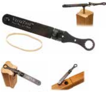
3044 Versa Tool Our VersaTool locates holes as well as starts and tightens hex nuts onto rail bolts. Drives 5/16" rail bolts and tightens 1/2" hex nuts. Also used to locate 1/4" pilot hole on handrails & rail drops for attaching to Connect-A-Kit® handrail fittings
