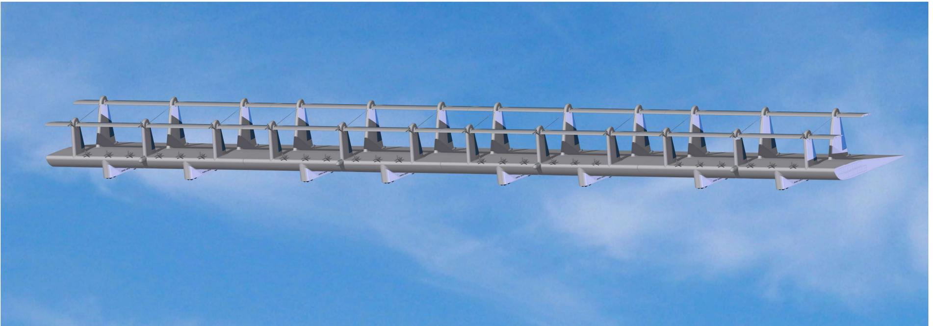
Folding wing extensions with additional tail plane, 260 ft span,
