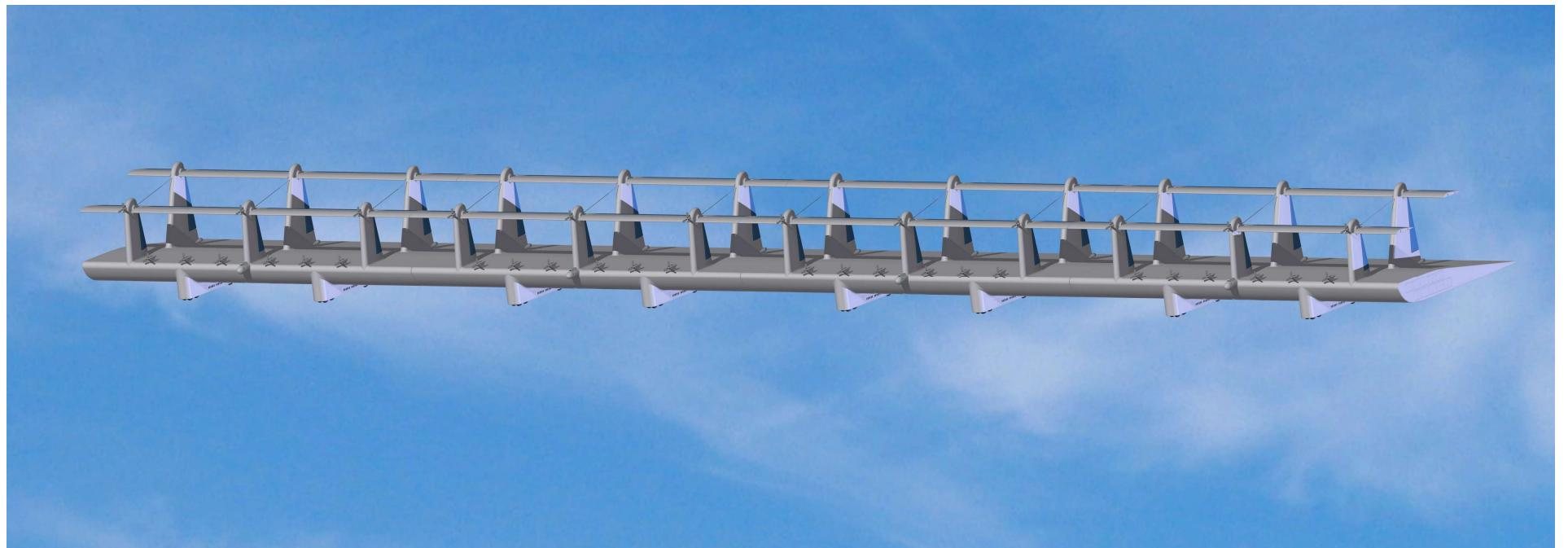
Folding wing extensions with additional tail plane, 260 ft span, 150 ft cord, 52 TEU or eight Abrams tanks.
