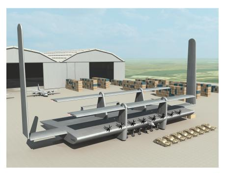
Cargo and auxiliary wings 260 ft. spans, total span of 700 ft. 69,300 sq. ft. of wing and a GWT of 1,396,000 lb.
