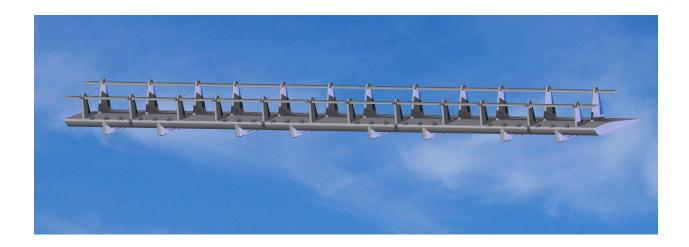
This has folding wing extension, and an additional tailplane. It could carry 52 TEU in 4 channels. The illustration below shows it with the wings folded. It could carry the eight Abrams tanks in front.
