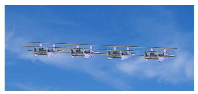
The next version, shown as a Ro - Ro, carries 320 automobiles in 20 channels. It could carry 78 TEU in 6 channels of 13 each. The cargo airfoil pod has a 200 ft. cord and fanjet exhausts for the boundary air system. The cargo wing and the auxiliary wings above have 260 ft. spans. It has 62,100 sq. ft. of wing. Using 20 lb. per sq. ft., it has a GWT of 1,242,000 lb. This could carry passengers and their automobiles across the Atlantic in 24 hours at low cost.
