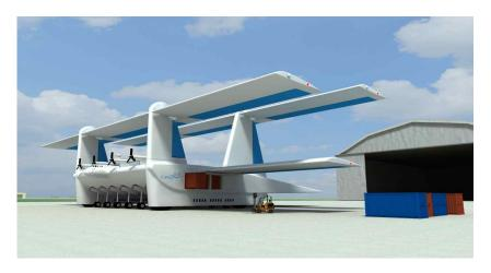
This version carries 20 TEU in 4 channels of 5 each. The cargo airfoil pod is 100 ft. wide with 80 foot extensions on both the cargo wing and the auxiliary wings above. It has 35,000 sq. ft. of wing. Using 20 lb. per sq. ft., it has a GWT of 708,000 lb. Windows and doors are shown for scale, however cargo ships used to carry a few passengers.
