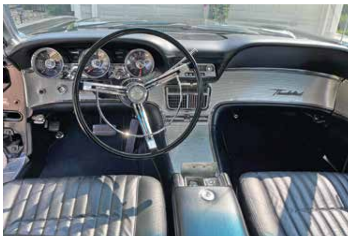
On Steve Cook's Thunderbird, a movable steering wheel cost $25.10. The steering wheel slides out of the way, to the right, allowing for better ease getting in and out of the car. Photo by Jackie Wilson
