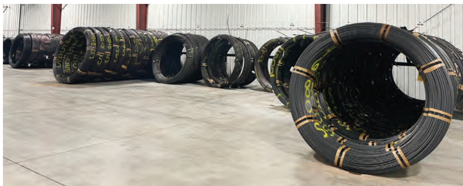
Steel wire spools provide the materials to make a variety of springs.
