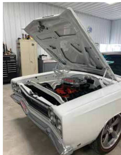
Jeff McCulley upgraded the engine to be more modern by using a late model 6.4 Liter Gen 3 Hemi in his 1968 Plymouth GTX.
