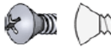
Oval A countersunk head with a rounded top. Abbreviated OH or OV
