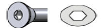
Socket, Hex or Allen A hexagonal hole for use with an Allen wrench.
