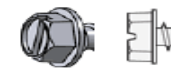
Slotted Hex Washer A hex head with built in washer and a slot.
