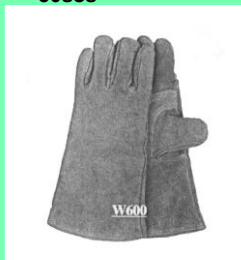
MEN'S WELDERS GLOVE SPLIT LEATHER, FIRE RESISTANT KEVLAR THREAD SEWN. FULLY SOCK LINED. REINFORCED THUMB 60861 GRAY WELDERS GLOVE 60863
