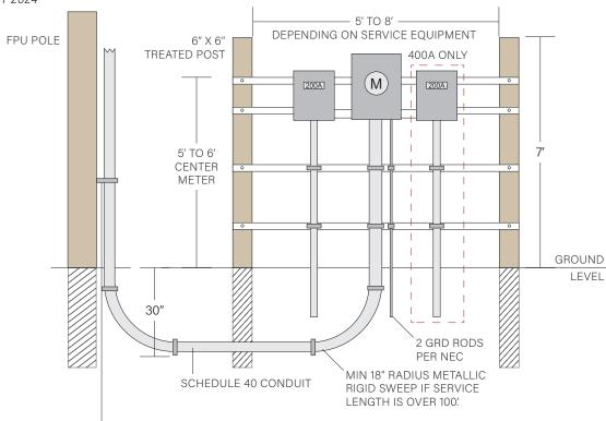
CONDUIT SET AT 3.5" OFF POLE, 3" SCH 80 AT POLE TO BE BROUGHT ABOVE GROUND LEVEL BY CUSTOMER.
