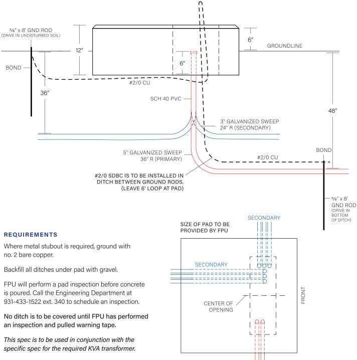
Contractor is responsible for verifying transformer dimensions and concrete pad dimensions will work together.
