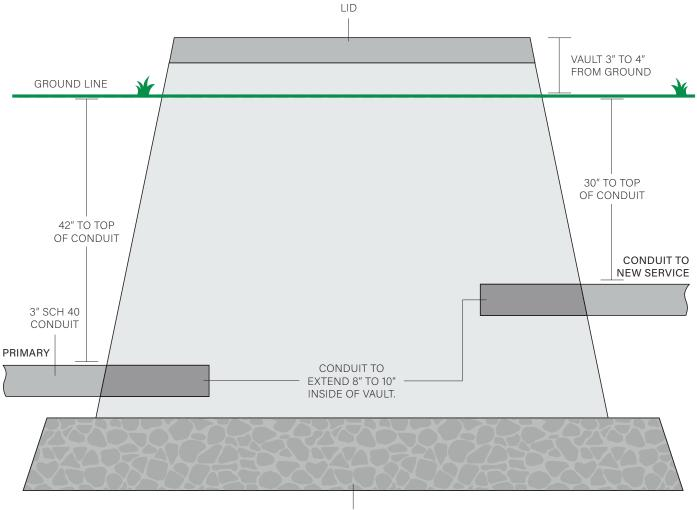
6" OF CRUSHED STONE UNDER VAULT
