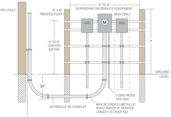
CONDUIT SET AT 3.5" OFF POLE. 3" SCH 80 AT POLE TO BE BROUGHT ABOVE GROUND LEVEL BY CUSTOMER.
