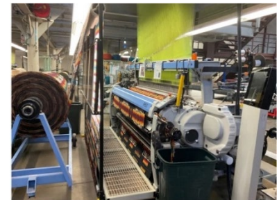
A Jacquard loom in action. This one has 250 harnesses.
