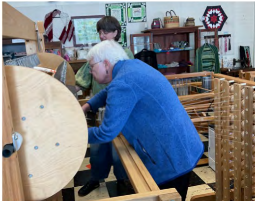
Winding on the sectional warp on the AVL
